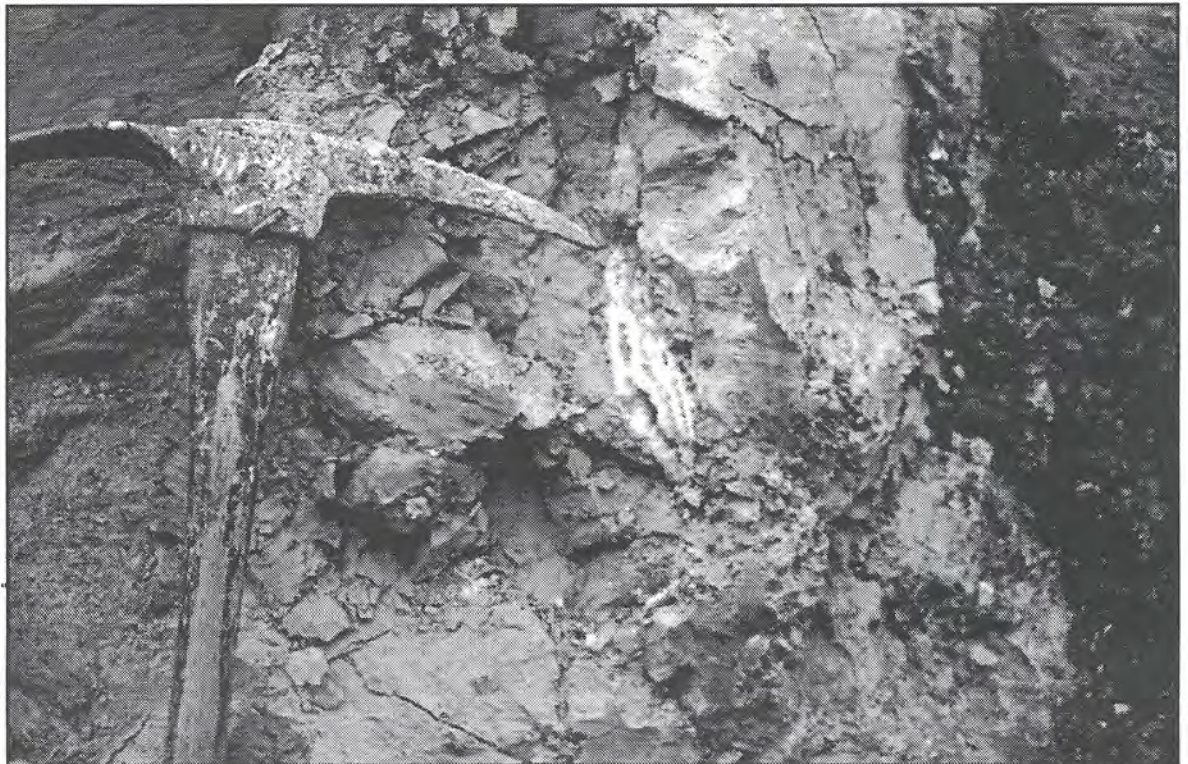
Figure 3. Crystalline calcite in fault plane shown at end of pick was radiocarbon dated, indicating that movement along the faults ceased by the Holocene.
