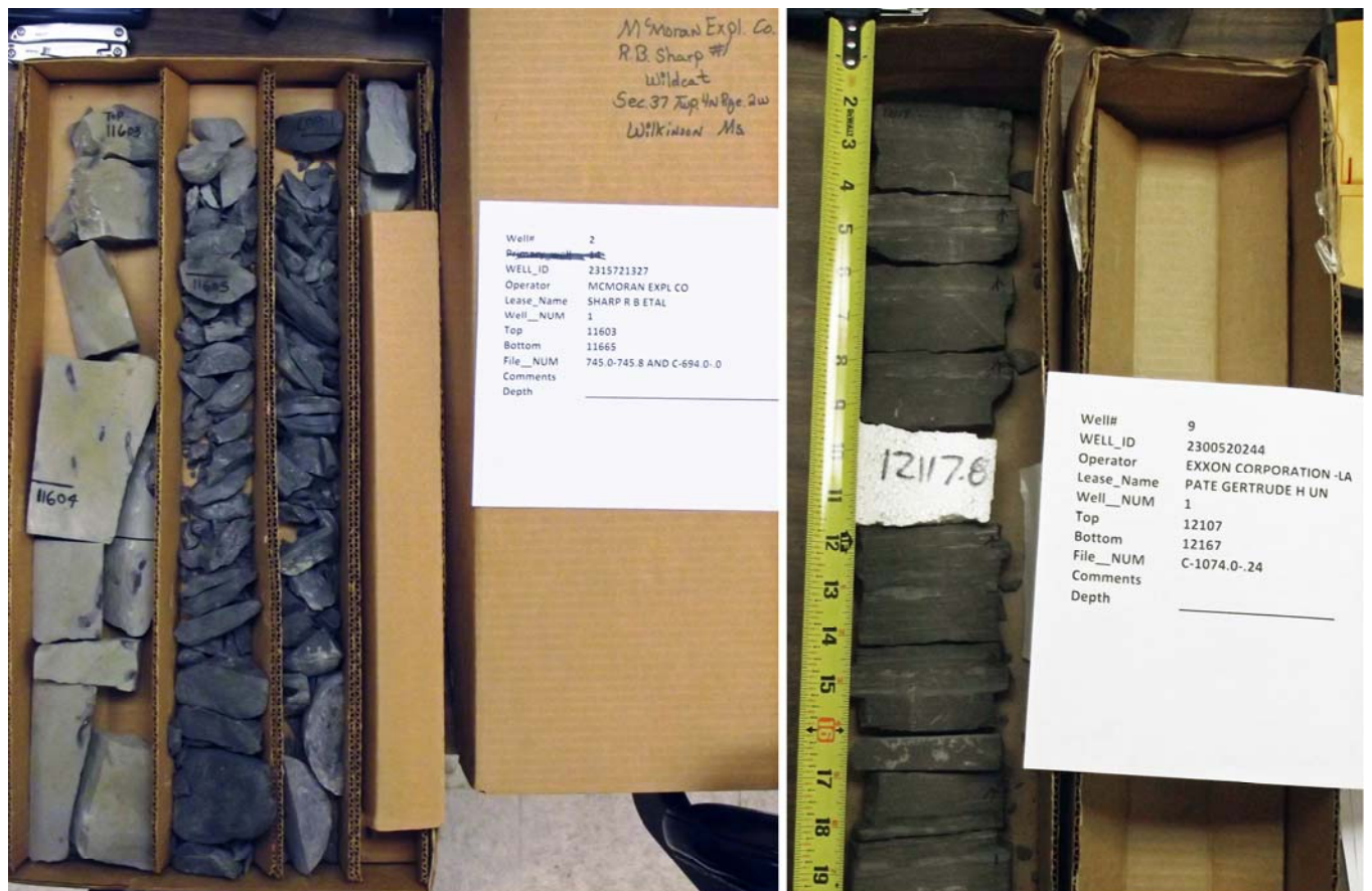
Figure 1. Cores from the Tuscaloosa marine shale sampled by the U.S. Geological Survey at MDEQ's Core and Sample Library in Jackson.
