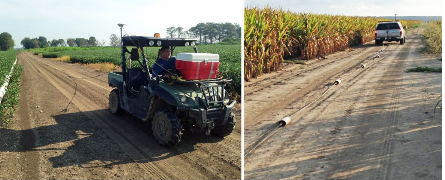
Figure 3. ATV pulling an array of electrodes for mapping in the vicinity of Steiner (left) and view of the Ohmmapper system in Sunflower County (right).
