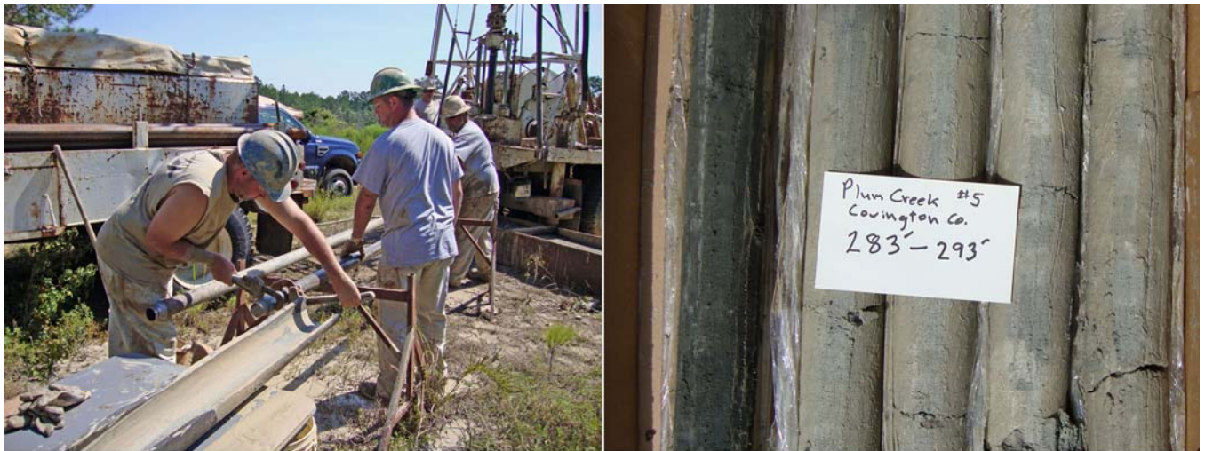
Figure 4. Left, left to right, James Starnes, Jonathan McKinnon, Trey Magee, and Archie McKenzie preparing to extrude a core from the Plum Creek #5 Covington core hole. Right, first core to contain the Heterostegina marine interval in the Catahoula Formation in Covington County.
