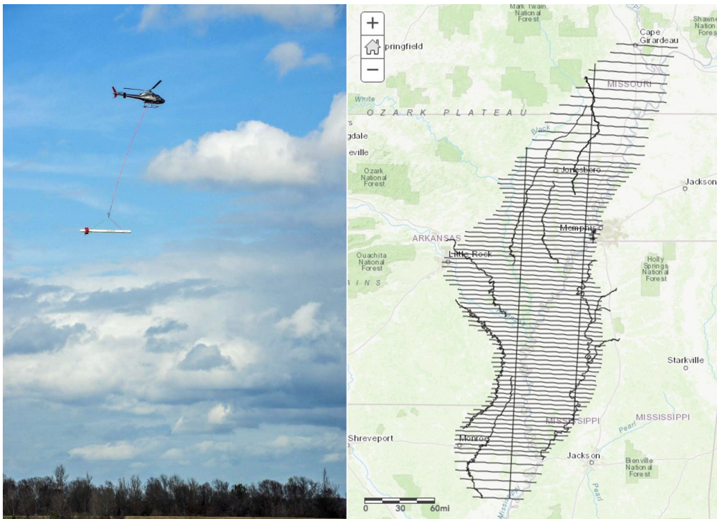
U.S. Geological Survey high-resolution airborne geophysical survey of the Mississippi River Valley Alluvial Aquifer.
