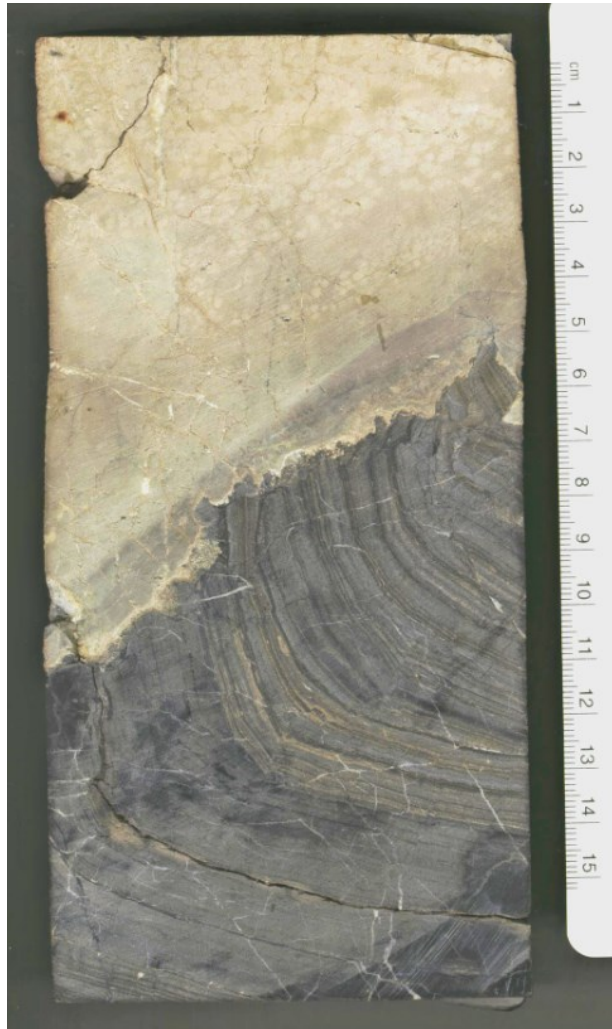
Figure 9. Deformed Smackover Limestone at the contact of a phonolite (71.6 Ma) intrusion in the Mississippi Valley Gas #1 Terry Bell in Washington County at a depth of 4,024 feet (MGS core box C-49.6). Picture made by James Starnes on a flatbed scanner; Image 813.
