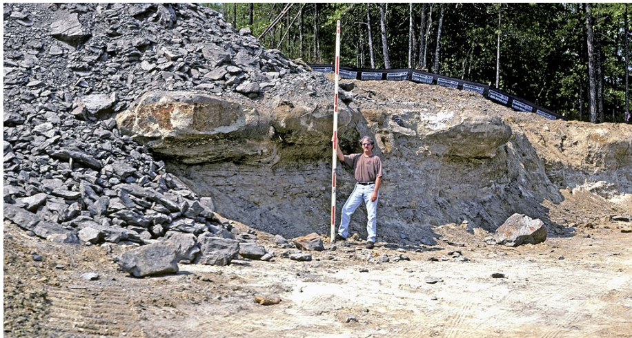
Figure 2. David Thompson holding survey rod at the contact of lowstand and overlying concretionary marine deposits in the Bashi Formation at the bridge construction site for the Walmart store in Meridian, Mississippi. To the left is shale excavated from the basal Hatchetigbee Formation. Picture was taken on August 18, 2000.
