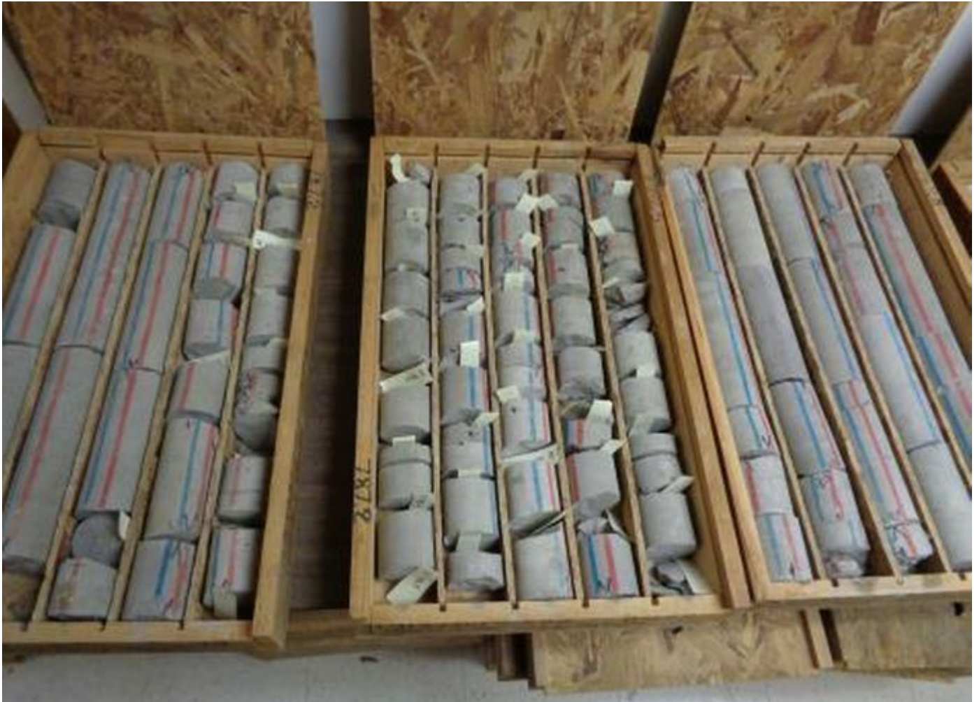
Figure 3. Cretaceous chalk cores from the Demopolis Formation at Shuqualak, Mississippi, in MDEQ's Core and Sample Library in Jackson.
