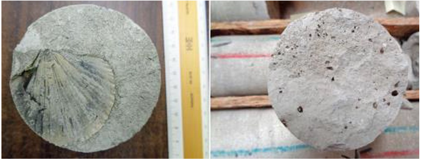
Figure 4. Bedding planes in the Cretaceous chalk core from Shuqualak, Mississippi, in MDEQ's Core and Sample Library in Jackson. At left is the fossil pecten Neithea quinquecostata and at right are biotite crystals (black) from a volcanic eruption at Jackson 75 million years ago.
